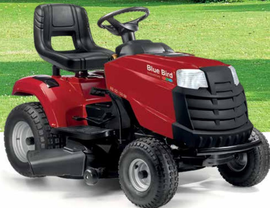
For all models, the cutting height is adjustable in 7 different positions, from 25 mm to 80 mm. The machines are equipped with hydrostatic transmission that allows complete speed control via a pedal for both forward and reverse. In addition, the activation of the blades takes place via an electromagnetic clutch by simply pressing a button.
